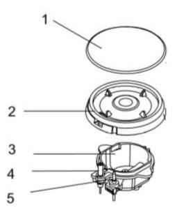
**NOTE:** Do not mix the top and bottom. The locating pins must fit exactly into the notches.
