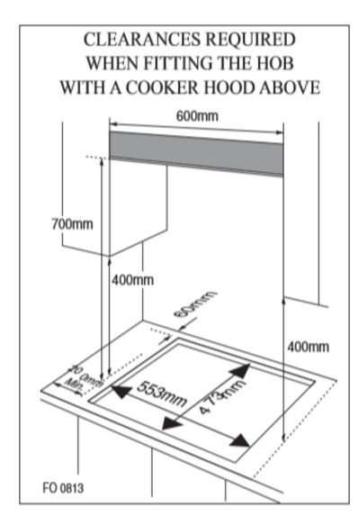
The edges of the hob must be a minimum distance of 60mm from a side or rear wall.
